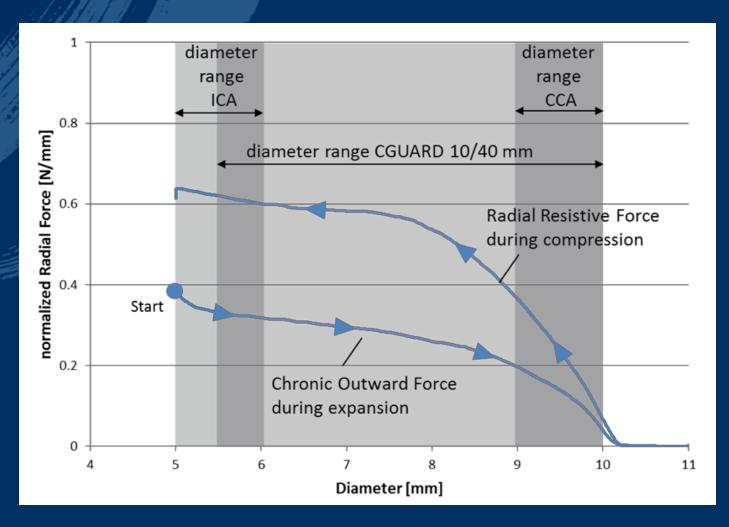
The chronic outward force, normalized by stent length, indicates a near-equivalent radial force between the minimal radial force at 9.0 mm (0.195 N/mm) and the maximal radial force at 5.5 mm (0.330 N/mm)
